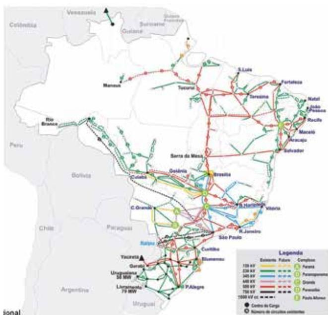
Figure 2. Brazil's power transmission grid, which could help fill the gap in midstream transport. Source: Sistema Interligado Nacional.
